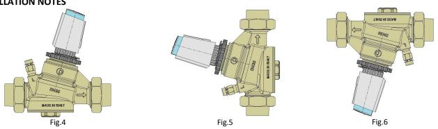
Vertical (Fig.4) or Horizontal (Fig.5) installation are recommended. An upside down (Fig.6) installation may reduce product life through special circumstances (i.e. contaminated water).
