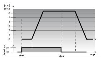
On this diagram is represented the characteristic line for the actuators A564O2 24V ON/OFF-PWM N.C. (Normally Close).
