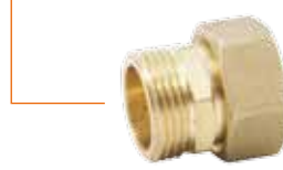
Union piece 3/4" F sphero conical x 1/2" M flat seat
