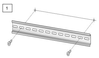
Install a DIN rail on-surface or in the heating circuit distributor cabinet.
