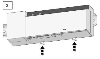
Fix the Base Station securely with the locking mechanism on the DIN rail.
