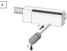
Remove the cover with a screwdriver.
