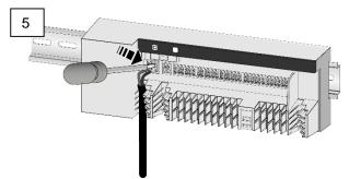
Lay the cable into the casing through the strain relief and install all cables to the Base Station using the clamping/plugin technology; this is possible in a very short time.
