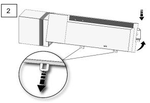
Position the base station slightly tilted onto the DIN rail and latch it in.
