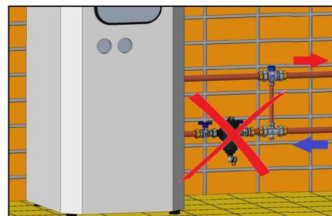
Upside-down and horizontal installation of the magnetic dirt separator **MUST BE AVOIDED**
