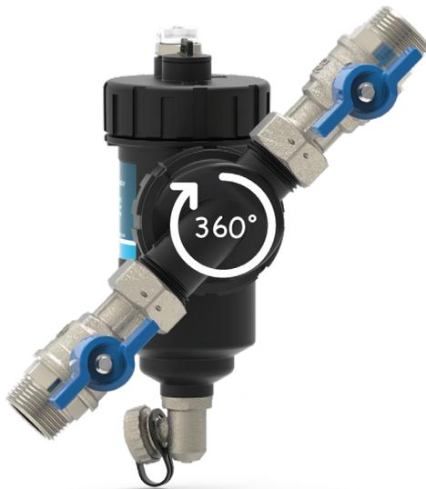
A specific feature of EvoMAGic 103 series is the orientable connection: despite the dirt separator has to work vertically, the 360° orientable connection allows the installation on different pipe direction. It can be installed on vertical, horizontal or tilted pipes. Installation requirements must be observed. Refers to specific INSTALLATION section.
